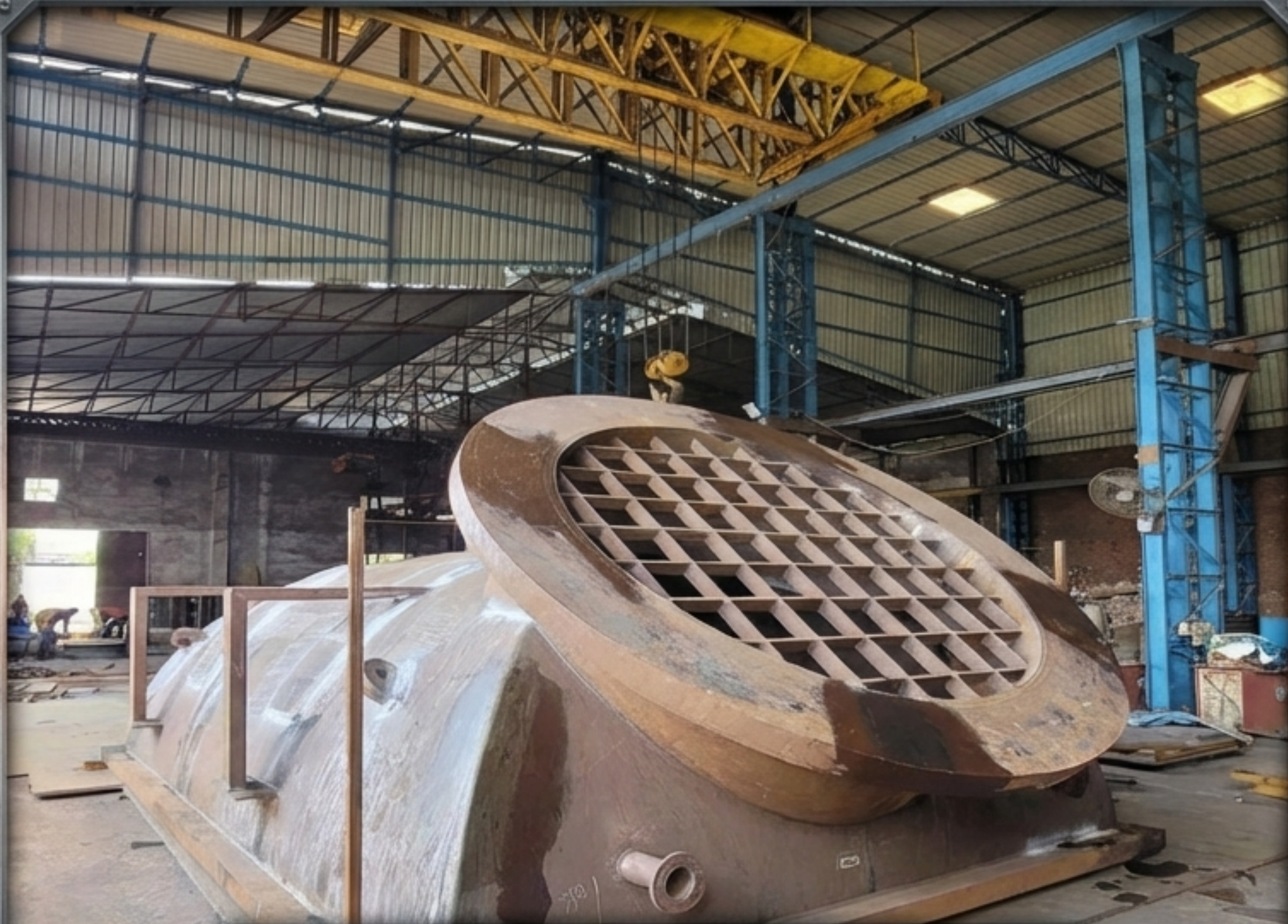
Handling heavy boiler and pressure vessel components with integrated lifting infrastructure.
